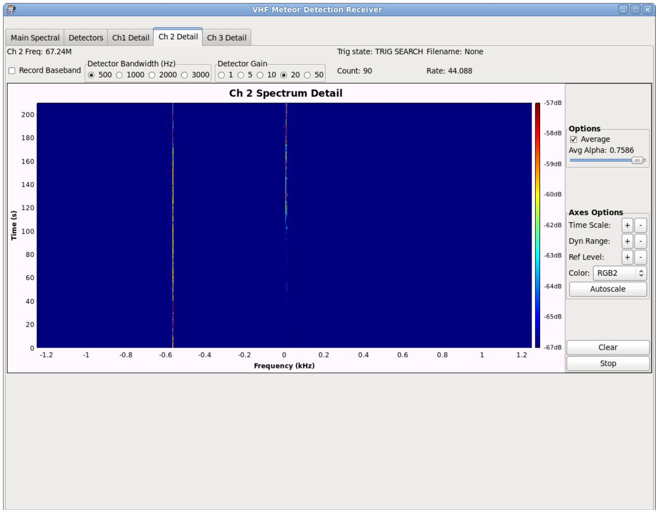
Above, we can see the tail end of an “event” near the middle, at 0Hz, and a local spur, offset almost -600Hz from the central carrier spectral component.
