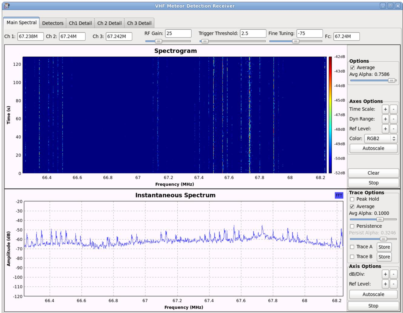
This shows the input 2MHz bandwidth, both as a conventional PSD spectrum, and as a colour-mapped spectrogram.
