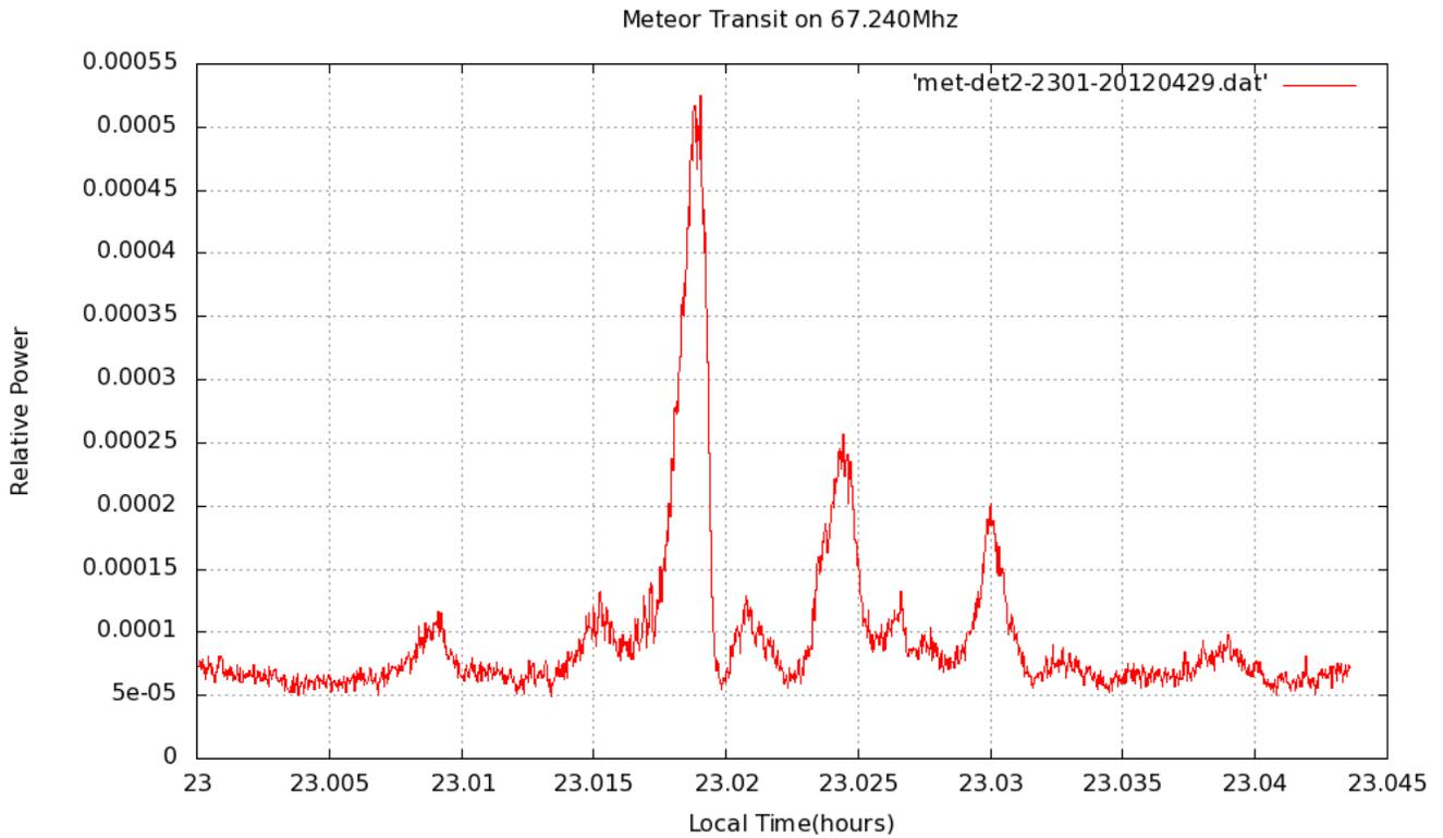
It's easy to see the large-timescale scintillation effects in the above event record, as the specular-reflective "surface" of the ionization trail causes changes in received power as the trail moves relative to the receiver.
