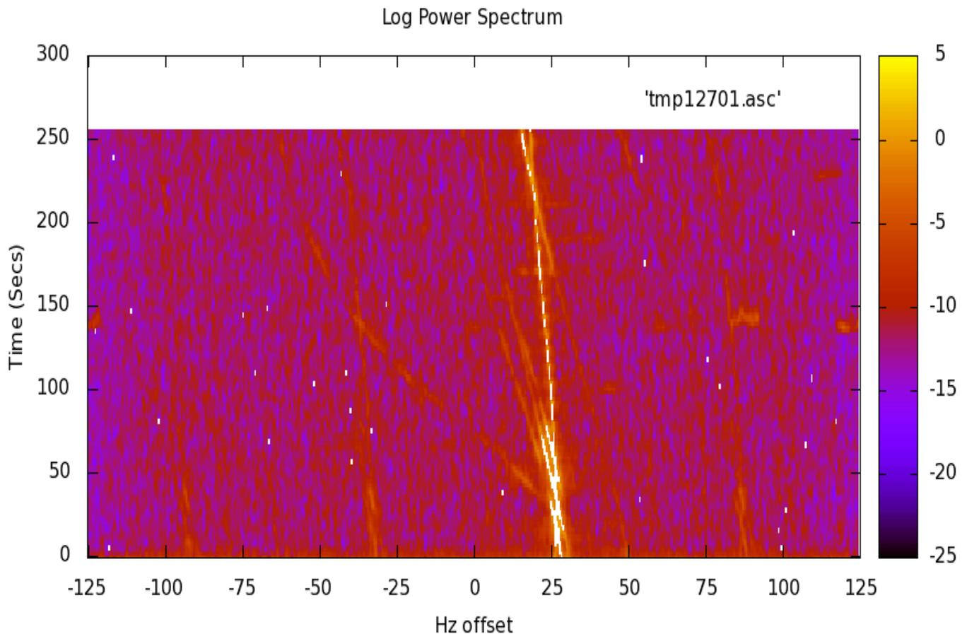
The above spectrogram shows several spectral features whose frequency changes over the course of the observation, and with further analysis can yield information about relative velocities. Weak 60Hz harmonic content is shown above for the first few 10s of seconds of the event, strongly suggestive of the video-carrier origins of this event. In fact, NTSC video signals have observable components at 60Hz and 15750Hz intervals (vertical refresh interval, and horizontal sync frequency respectively).
