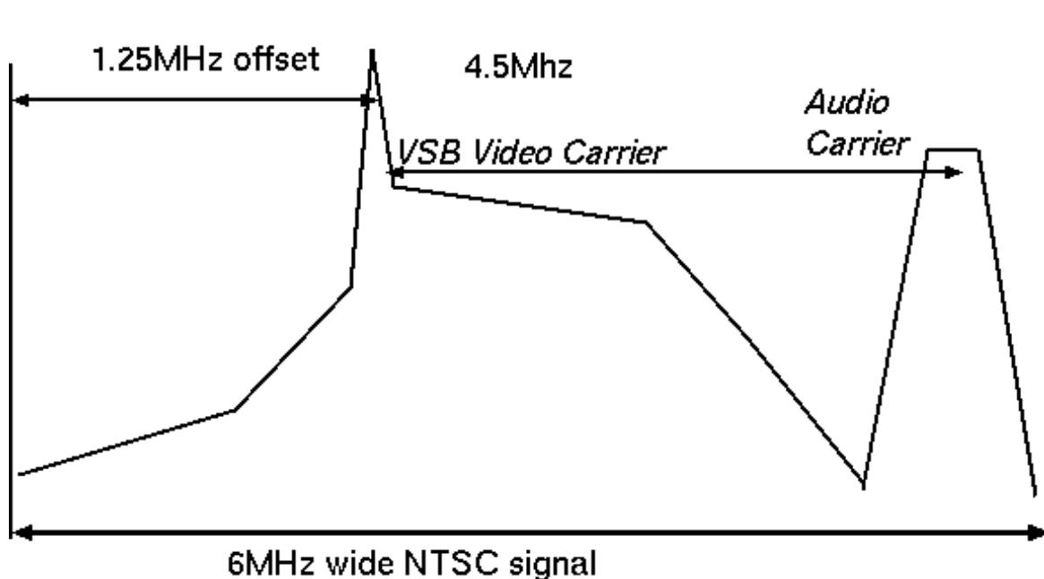
Note that the video carrier is VSB modulated, which is similar to AM, but with the lower sideband significantly attenuated to save bandwidth. The central spectral component in the VSB carrier tends to be stronger than the other components, and quite stable. So this component can easily be used to measure Doppler signatures of an analog TV signal that is scattered by a meteor event.
