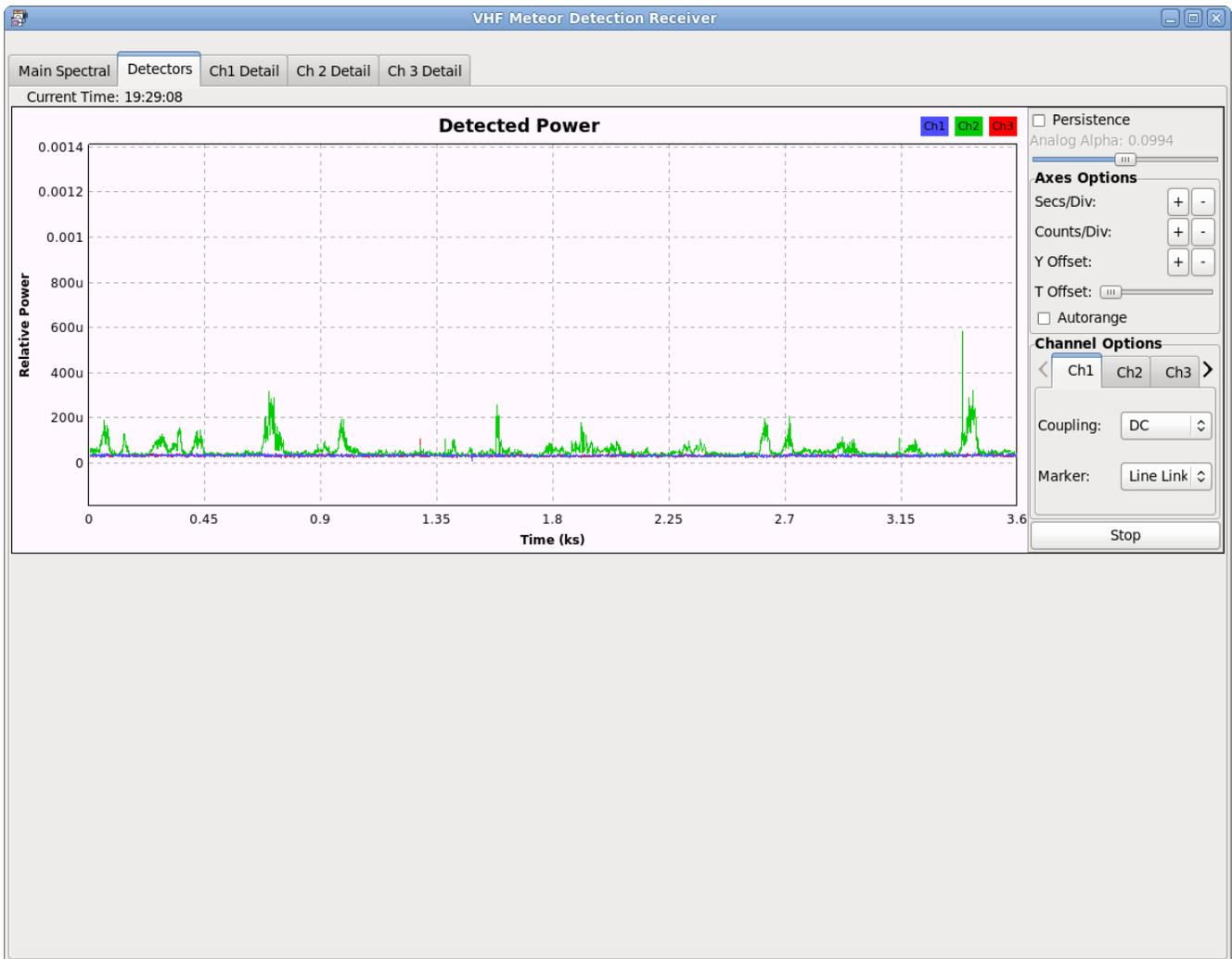
Shown above, we can see that the central channel, in this case tuned to the TV channel 4 video carrier at 67.240Mhz (shown in green above) contains several significant events, whereas the “check” channels either side of the central channel have no such events shown, which is precisely what is to be expected using a TV video carrier.
