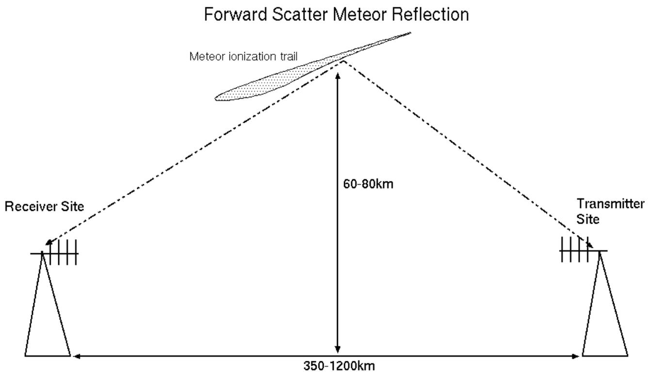
Path lengths of 350-1200Km are typical. Below 350km, the direct, tropospheric, path can interfere with detections from the forward-scattered signals.
